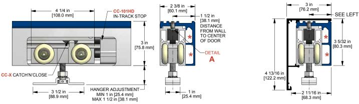
[CC-902 Side Mount Bracket illustrated as solid blue profile. Supplied in continuous lengths.] [\*Indicates mounting locations to the wall support on CC-902 Side Mount Bracket] [Optional CC-920 Snap-On Fascia illustrated as solid black profile]
