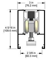
[Optional CC-940 Snap-On Fascia illustrated as solid black profile. Can be used on both sides of the track or one side only]
