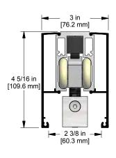
[Optional CC-940 Snap-On Fascia illustrated as solid black profile. Can be used on both sides of the track or one side only]
