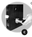
C. With outside lever/knob in the horizontal orientation, carefully insert the mounting posts through the door and lockbody, making sure the spindle is engaged in the lock. Outside rose assembly should be flush with door surface.
