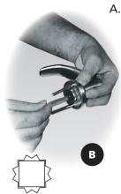
A. With outside rose assembly in hand tighten the retaining nut against the mounting plate as far as it will go by hand. To insure a tight fit in this assembly, back off retaining nut just one notch, until star pattern lines up with square corners. (see pattern shown)
