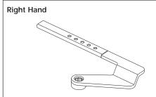
For double egress doors with reveal greater than 1/8" (3mm) and less than 3" (76mm)
