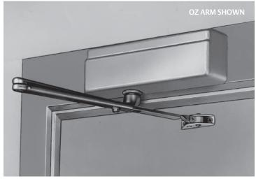
Top Jamb applications - The 1431 closer is mounted on the frame face above the door. The foot is mounted on the push side of door. This application is for use on exterior doors opening out to protect the closer from the weather.
