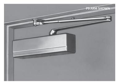
Parallel Arm Applications - The 1431 closer is mounted on the push side of the door with the arm under the frame parallel to the face of the door. This application is well suited for narrow face frames and deep reveal applications. The closer arm does not project into the room, and the door can be swung open much farther than in Top Jamb Application.
