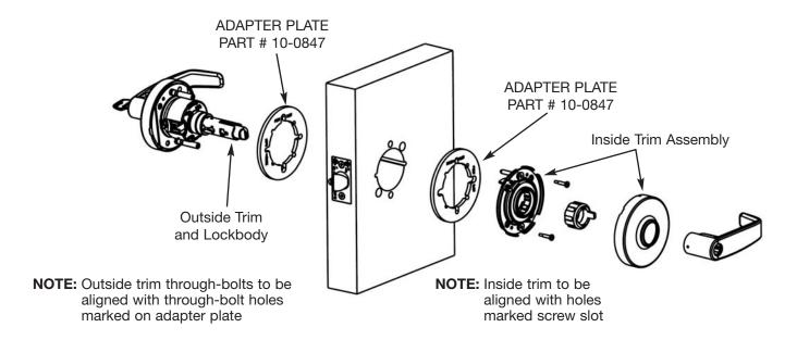
Install (1) adapter plate between door and rose assemblies (both sides) For lock installation, refer to instruction sheet A7133G
