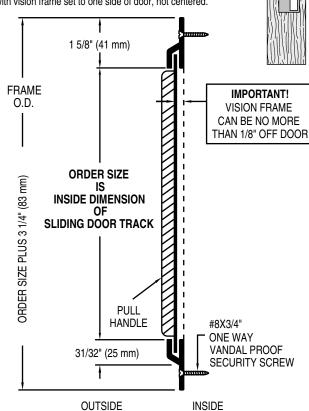
NOTE: When used with vision frame other than LoPro. or SG-10 outside dimensions of frame must be furnished.
