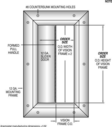
NOTE: Door slides from side to side. Non-centered vision frame cutout is generally required, i.e. 12" x 12" LoPro vision frame requires 26" x 13' SSD with vision frame set to one side of door, not centered.
