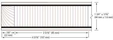
Two 1/32" (0.8 mm) or 1/16" (1.6 mm) lead sheets bonded to the core
