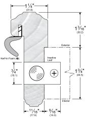
$(\frac{5}{16}"$  diameter  $\times$  1" long throw bolt) and one  $\frac{1}{2}"$  thick sponge neoprene bottom seal with double faced adhesive for attachment (non-handed)
