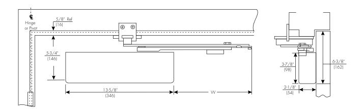
Mounting holes for closer body are spaced 2-3/8" (86mm) vertically  $\times$  6-3/4" (171mm) horizontally. Door width must be specified when ordering.
