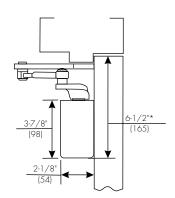
Mounting holes for closer body are spaced 2-3/8" (86mm) vertically x 6-3/4" (171mm) horizontally. \* This dimension will vary. Standard non-hold open arm illustrated.
