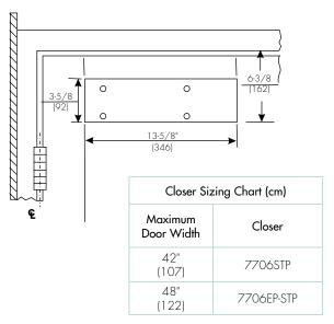
7706STP or 7706EP-STP Series Closers Slide Track for 90° Wall Pocket Installation For Pocket Depths 2-1/4" to 4-1/4" (57mm to 108mm) (See Chart for Closer Sizing)
