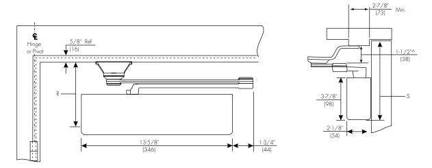
Mounting holes for closer body are spaced 2-3/8" (60mm) vertically x 6-3/4" (171mm) horizontally. ^ If clearance greater than 1-1/2" is needed, 6891 spacer block is required.
