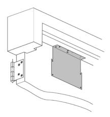
Metal templates help the installer locate the correct mounting holes for several parallel arm applications.
