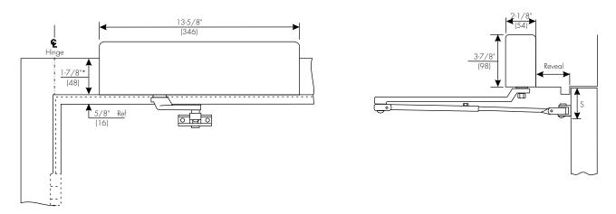
Mounting holes for closer body are spaced 2-3/8" (86mm) vertically x 6-3/4" (171mm) horizontally. \* Minimum frame face with 7786 drop plate. 3-1/4" (83mm) required when drop plate is not used.
