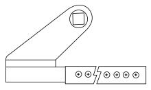
Arm Tube Assembly 7701ST-1ATR<sup>1</sup> (right hand) 7701ST-1ATL<sup>1</sup> (left hand)
