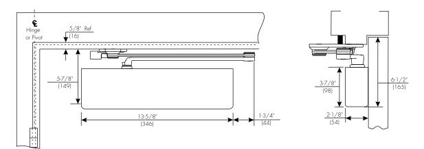
Mounting holes for closer body are spaced 2-3/8" (60mm) vertically  $\times$  6-3/4" (171mm) horizontally.
