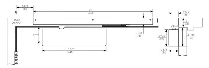
Mounting holes for closer body are spaced 2-3/8" (86mm) vertically x 6-3/4" (171mm) horizontally.
