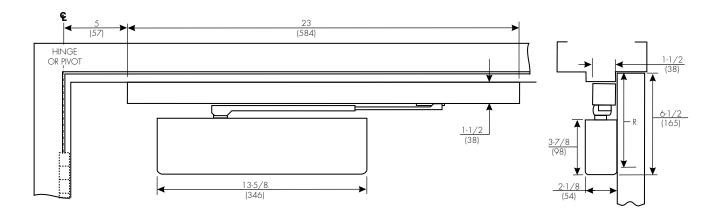
Mounting holes for closer body are spaced 2-3/8" (86mm) vertically  $\times$  6-3/4" (171mm) horizontally.
