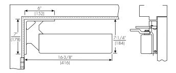
Mounting Opposite Hinge Side - #7798 Standard Drop Corner Bracket: For use where it is desired to mount a regular arm non-hold open closer.
