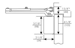
Mounting holes for closer body are spaced 2-3/8" (60mm) vertically  $\times$  6-3/4" (171mm) horizontally.
