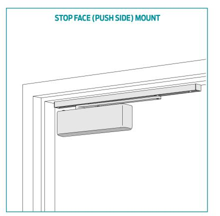
The 4210T SMOOTHEE® Series is a heavy duty, high security track closer with special components to minimize tampering and vandalism. Forged steel arms and heavy gauge metal security covers are designed for correctional, vandal prone, institutional and other high traffic interior applications. The closer has passed 10 million cycles in independent testing. A choice of finishes and cylinder functions meet correctional and vandal resistant requirements.
