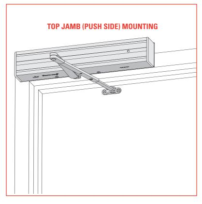
The 4410ME SENTRONIC® is a heavy duty, electrically controlled closer/holder designed to provide infinitely adjustable hold-open for fire and smoke barrier doors.
