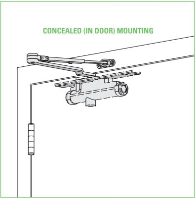
The concealed 3030 is designed to mount in a 1 3/4" interior door. The double lever arm provides superior door control and the choice of finishes and arm functions meet virtually all architectural requirements.
