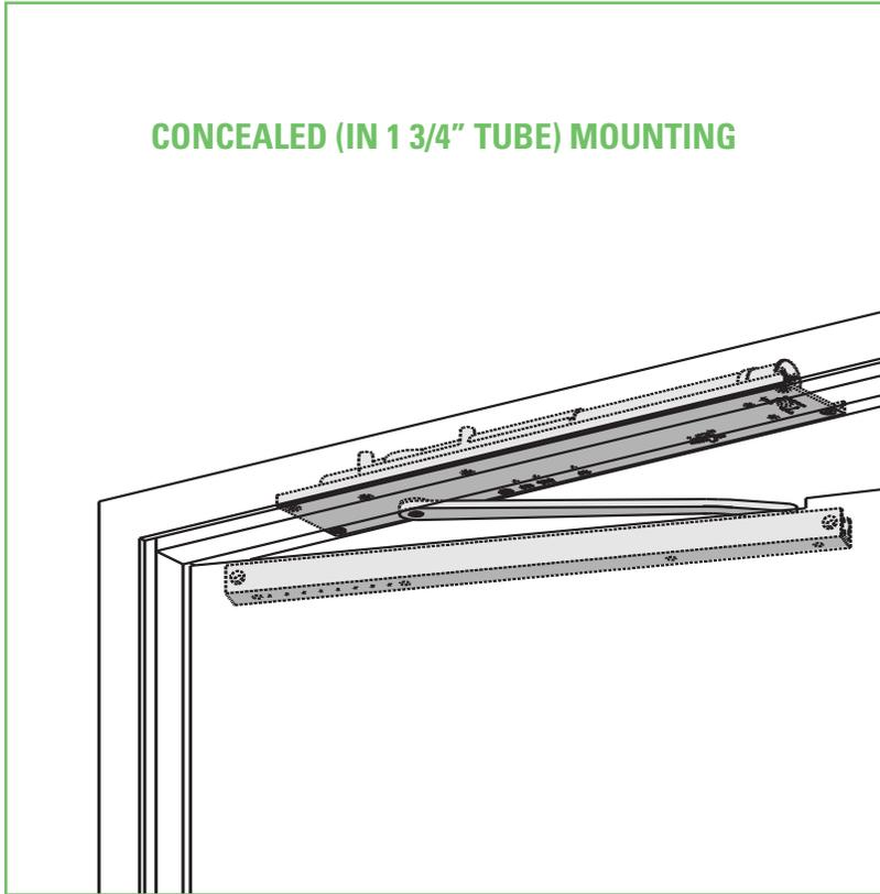
*The concealed 2030 Series PACER® is a heavy duty closer designed to fit in a narrow, minimum 1 3/4" aluminum transom. The single lever arm and roller assembly provide smooth, quiet door control and the choice of finishes and track functions meet virtually all architectural requirements.*
