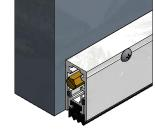
**SURFACE MOUNTED:** FITS BETWEEN STOPS. (ALLOW 1/16" CLEARANCE AT BOTH ENDS BETWEEN HOUSING AND STOP).
