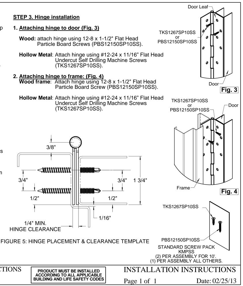
All holes in the doors and frames must be drilled correctly and fasteners properly installed. Failure to use the fasteners supplied by Markar Architectural Products will void the UL or WHI fire rated listing.
