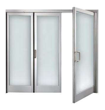
The easy-to-install DORMA ICU1200 is a perfect fit for installations with limited width and self-closing requirements. The ICU1200 combines two types of door: a double-acting swing door on one side and a bi-fold manual door on the other. Narrow stiles and an optional muntin ensure clear views for observing patients. For normal traffic, the swing door conveniently opens in either direction. For a wider opening, the bifold door collapses to open up nearly the full width of the doorway.
