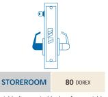
Latchbolt operated by key from outside or by inside knob or lever. Outside knob or lever is always locked. Auxiliary latch deadlocks latchbolt.
