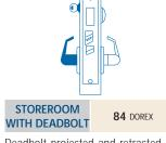
Deadbolt projected and retracted by key from outside or by inside lever or knob or thumbturn. Inside lever or knob retracts both bolts simultaneously. Extended deadbolt automatically deadlocks latchbolt.
