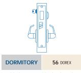
Latchbolt operated by knob or lever from either side or key from outside. Deadbolt projected/retracted by key from outside and thumbturn from inside. Deadbolt retracted by key from outside. Rotating inside lever retracts both bolts simultaneously. Extended deadbolt automatically deadlocks latchbolt.
