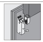
Contrary to the other door checks the R 1400 door damper is always mounted on the "back" of the door. Important: The R 1400 door damper should always be mounted at the side, approx. 8 mm from the closing edge as the hook reaches into the doorway. You can either fix the door damper horizontally or vertically.
