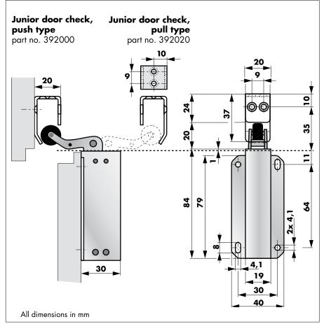
The door damper Junior pull type and push type just differ in the position of the operating lever with the rubber roller. The pull type has the operating lever fixed in the posterior holes of the casing and shows backwards (see dotted drawing). This type is used e.g. when the door damper is fixed to the back part of a drawer and the hook is fixed to the inner panel of the cupboard.
