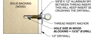
5/8"Ø X 1/2" ALUMINUM SPACER IS TO BE INSTALLED BETWEEN THREAD INSERT AND WALL MOUNT BRACKET. THIS WILL KEEP INSERT SEATED AND PREVENT
