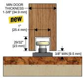
CUT C-914 ALUMINUM GUIDE CHANNEL TO CORRECT LENGTH IF REQUIRED (TYPICALLY, LENGTH EQUALS DOOR WIDTH. EXAMPLE: DOOR WIDTH IS 36" THEREFORE CHANNEL IS 36".) STEP 2
