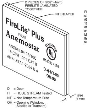
PLEASE NOTE: On visible lite sizes larger than 1296 sq. in. (0.836 m²) on 20/45 min. and 100 sq. in. (0.065 m²) on 60/90/180 min., please consult with your Door / Frame Manufacturer's procedures, for their maximum glass size tested.
