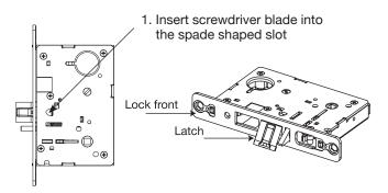
Rotate screwdriver 90° to push latch out until back of latch clears lock front. Then rotate latch 180°. Latch will then re-enter lockbody. (Note: Latch can not be unscrewed)
