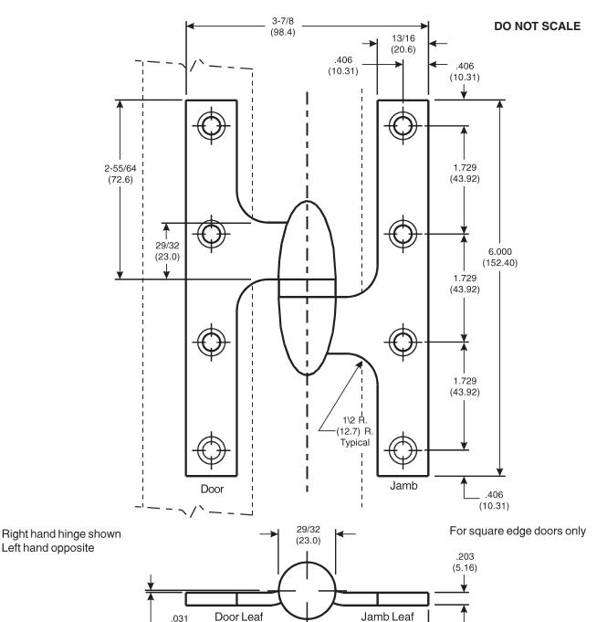
McKINNEY Template Olive Knuckle Hinges are made in size, gauge and with screw holes located to conform to this drawing. Machine Screw Size -  $1/2 \times 12-24$  F.H.
