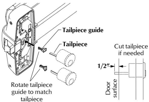
**7** Install trim (if using) and secure device center case to door.
