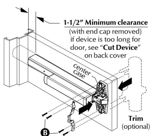
**8** Install mounting bracket and end cap.
