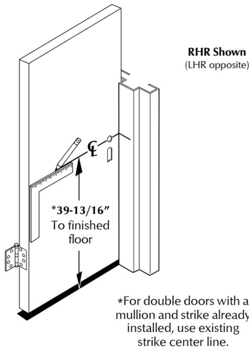
**2** Align strike on ☿ and mark the two slotted holes.
