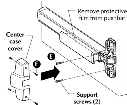
For 98F/99F (fire rated) devices on wood or composite door:
