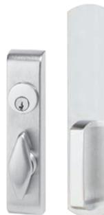
Standard operation, key locks and unlocks thumbturn. Optional operation, key unlocks thumbturn, re-locks when key is removed. This operation is created by changing the cylinder plate included with control. Use 1 1/4" mortise cylinder with a straight cam. Schlage cam reference B502-191. Use with a pull trim (990DT pictured).
