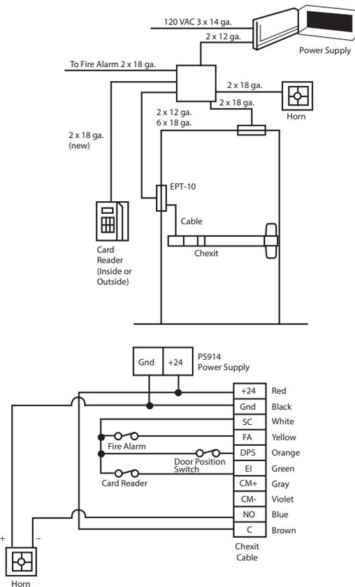
Chexit Single Door with Options – The Chexit is used as an access control device. The card reader allows access. Also shown in this application is an external horn and door position switch. The auxiliary horn is used for increased volume in remote locations. Using a door position switch gives added security to the opening in case the door is not reclosed.
