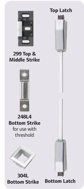
**9857/9957 three-point latching device** for all types of single or double doors, UL listed for Panic Exit Hardware. Devices are ANSI A156.3 – 2001 Grade 1. Covers stock hollow metal doors with 86 or 161 cutouts. The 9857 device has a smooth mechanism case and the 9957 device has a grooved case. The three-point latching device is non-handed except when the following device options are used: SD (Special Dogging), or SS (Signal Switch). See Opposite page for available outside trim and functions.
