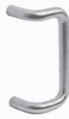
The 392-7 Offset Pull is 3/4" round stainless steel, with a 7" center to center which matches the 98/99 center case. Often used with a night latch operation. 3 1/2" (89mm) offset with 1 1/2" (38mm) clearance.
