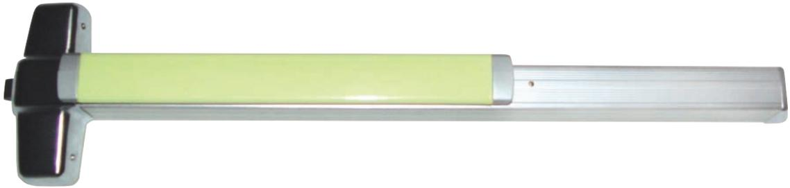
Self-illuminating touchpad defines the location of the exit door in dark or smoke-filled area. The Safety Glow coating is a special powder coat finish that glows brightly during low or no light conditions. This coating was developed to meet MEA standards where luminescent exit door markings are required in commercial facilities. There are no batteries or electronics, the coating is charged when exposed to light.
