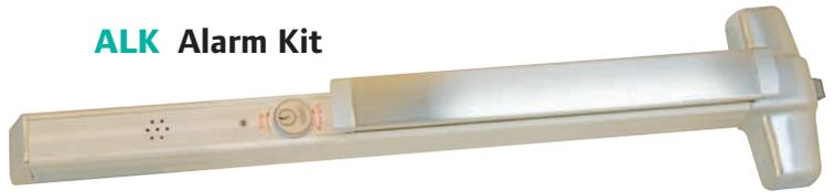
The ALK battery alarm kit is a simple yet effective way to deter unauthorized use of an opening. While the exit device is still a means of egress, the ALK kit contains an internal horn. When the touch bar is depressed, the horn sounds to provide an audible means of signaling that the opening has been violated. The alarm kit can be armed or disarmed by key. The horn is rated at 85 decibel.
