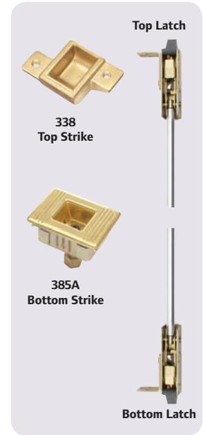
**9847/9947 concealed vertical rod device** for use on single or double metal doors, UL listed for Panic Exit Hardware. Devices are ANSI A156.3 – 2001 Grade 1. The 9847 device has a smooth mechanism case and the 9947 device has a grooved case. The concealed vertical rod device is non-handed except when the following device options are used: SD (Special Dogging), or SS (Signal Switch). See Opposite page for available outside trim and device functions.
