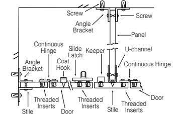
Standard gaps are provided at all walls and between components to allow for hardware attachment.
