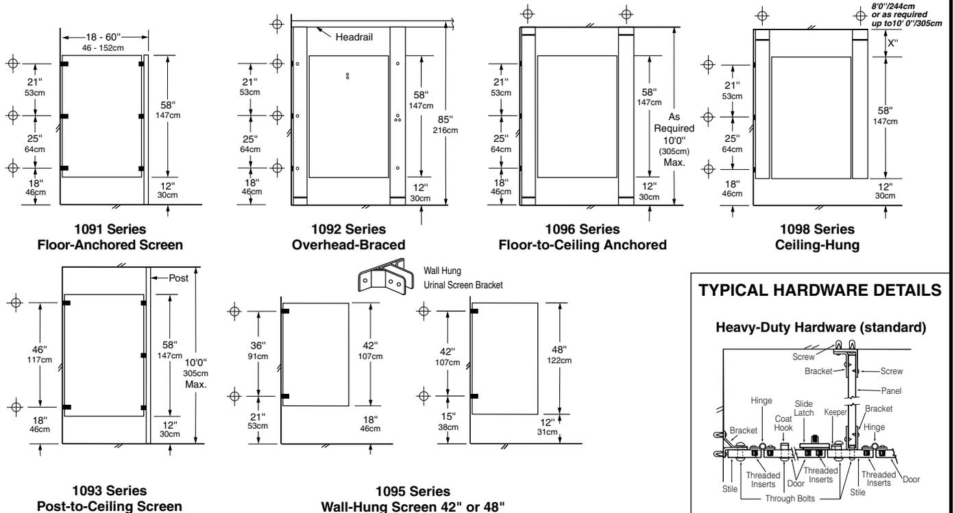
⊕ These mounting points require backing. For suggested backing methods, Bobrick Advisory Bulletins TB-32 for ceiling-hung installations and TB-66 for floor-anchored are available upon request.
