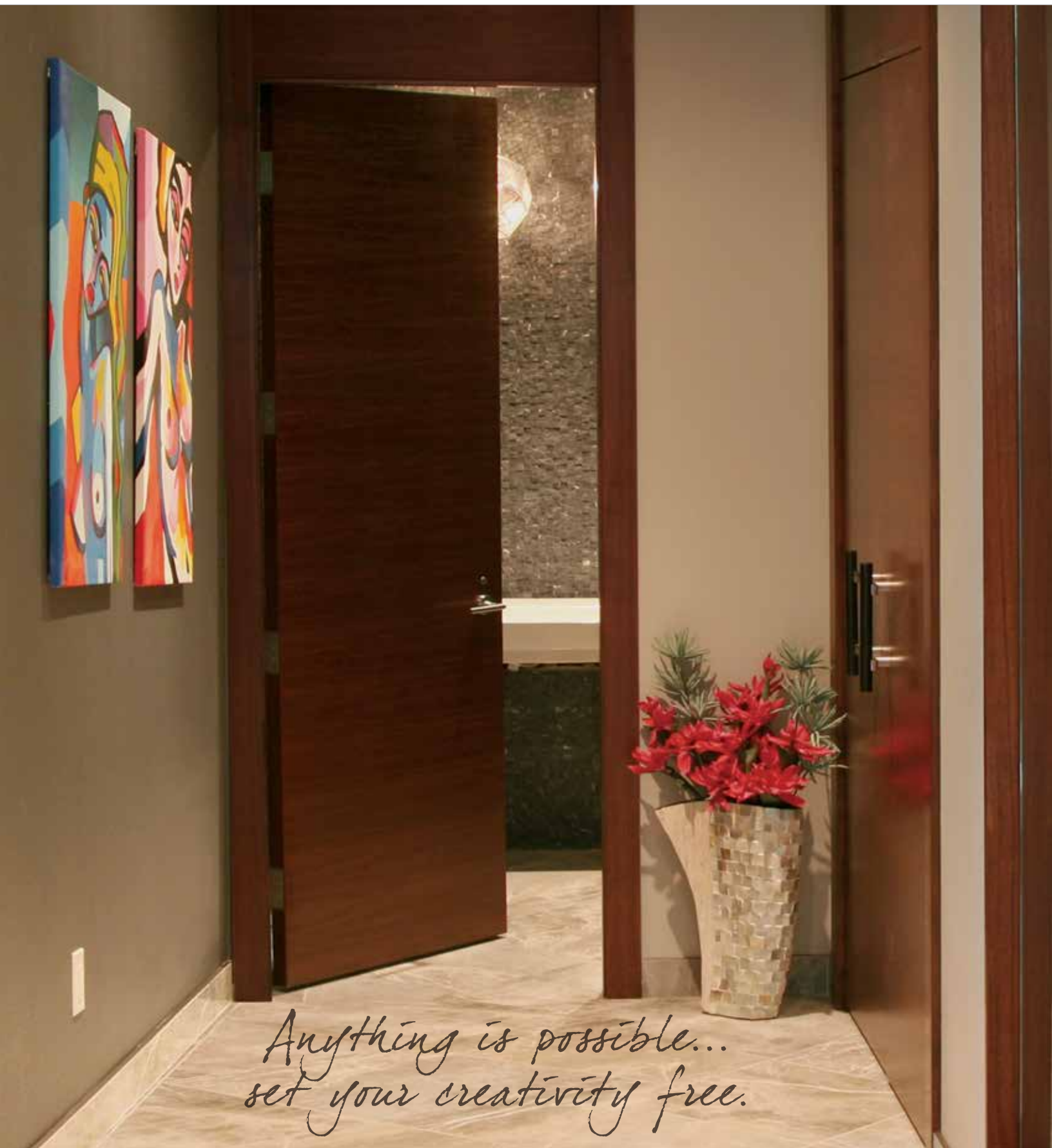
8 foot horizontal grain walnut flush door with matching transom and rabbeted walnut frame; Schlage L9060 mortise privacy lockset with Danmark lever in Satin Stainless Steel
