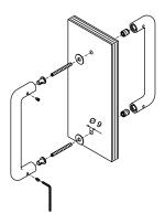
For installing a pair of pull handles without screw covering rosettes on a glass door, thickness 8-12 mm, for items.
