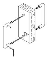
For installing a pair of pull handles without screw covering rosettes on a wooden door, thickness 45-55 mm 55-65 mm, for items.
