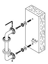
For installing a single pull handle with screw covering rosettes on a wooden door, or on a masonry wall using a brass anchor screw, for items.
