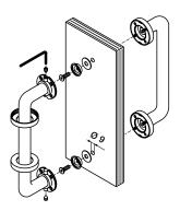
For installing a pair of pull handles with screw covering rosettes on a glass door, thickness 8 -12 mm, for items.
