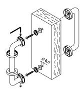
For installing a pair of pull handles with screw covering rosettes on a wooden door, thickness 45 - 55 mm 55-65 mm, for items.
