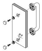
For installing a single pull handle with screw covering rosettes on a glass door, thickness  $8\,$  -12 mm, for items.
