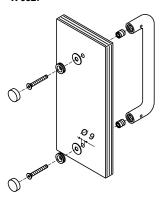
For installing a single pull handle without screw covering rosettes on a glass door, thickness 8 -12 mm, for items.
