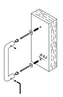
For installing a single pull handle without screw covering rosettes on a wooden door, or on a masonry wall using a brass anchor screw. for items.
