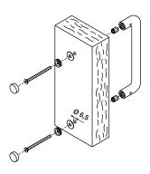
For installing a single pull handle without screw covering rosettes on a wooden door, thickness 45-55 mm 55-65 mm, for items.
