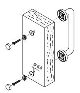
For installing a single pull handle with screw covering rosettes on a wooden door, thickness 45 - 55 mm 55-65 mm, for items.
