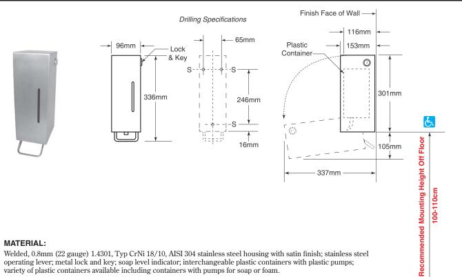
Welded, 0.8mm (22 gauge) 1.4301, Typ CrNi 18/10, AISI 304 stainless steel housing with satin finish; stainless steel operating lever; metal lock and key; soap level indicator; interchangeable plastic containers with plastic pumps; variety of plastic containers available including containers with pumps for soap or foam.
