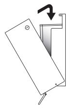
3. Ensure both top and bottom of container are correctly seated in dispenser.
