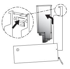
B. Press locking latch and lift cartridge up and out.
