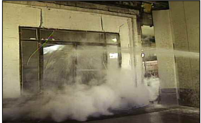
Fire hose impacting fire rated glass immediately after fire test.
